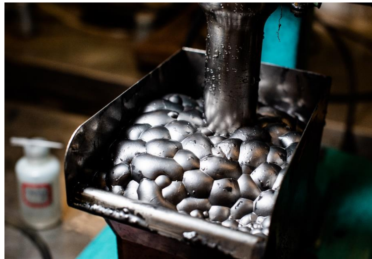
A laboratory scale froth flotation unit is used to separated anode powders from cathode powders. Courtesy of Michigan Technological University
